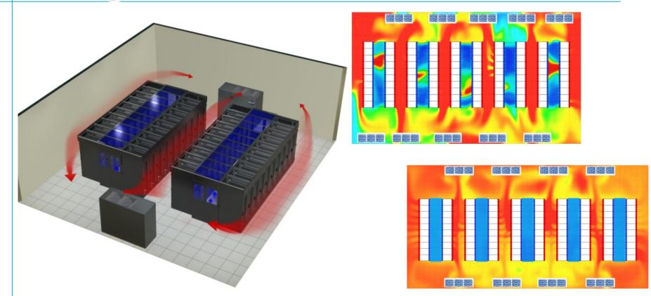
Hot-aisle/cold-aisle arrangement creates the opportunity to further increase cooling unit capacity by containing the cold aisle
