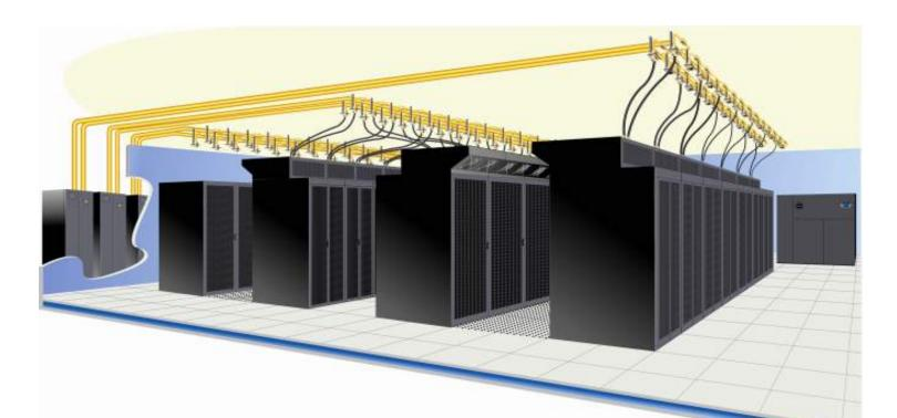
Refrigerant-based cooling modules mounted above or alongside the rack increase efficiency and allow cooling capacity to be matched to IT load.
