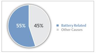
Figure 1. Battery-related failures account for more than half of all UPS system failures.
