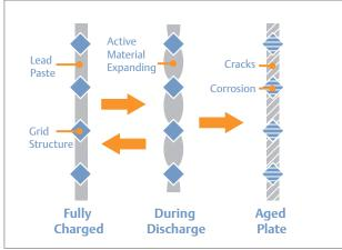
Figure 3. Batteries age when mechanical stress causes grid expansion.
