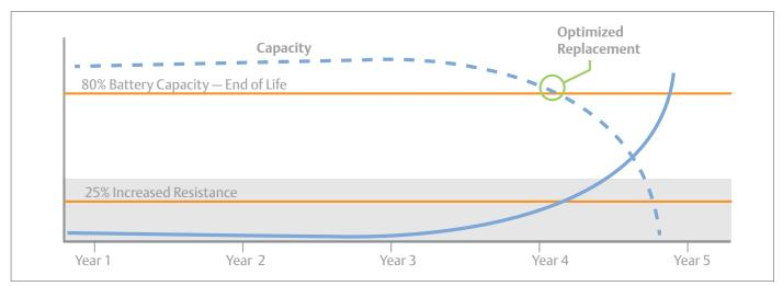
Figure 5. Batteries lose capacity as they age justifying the need for a preventive maintenance program.
