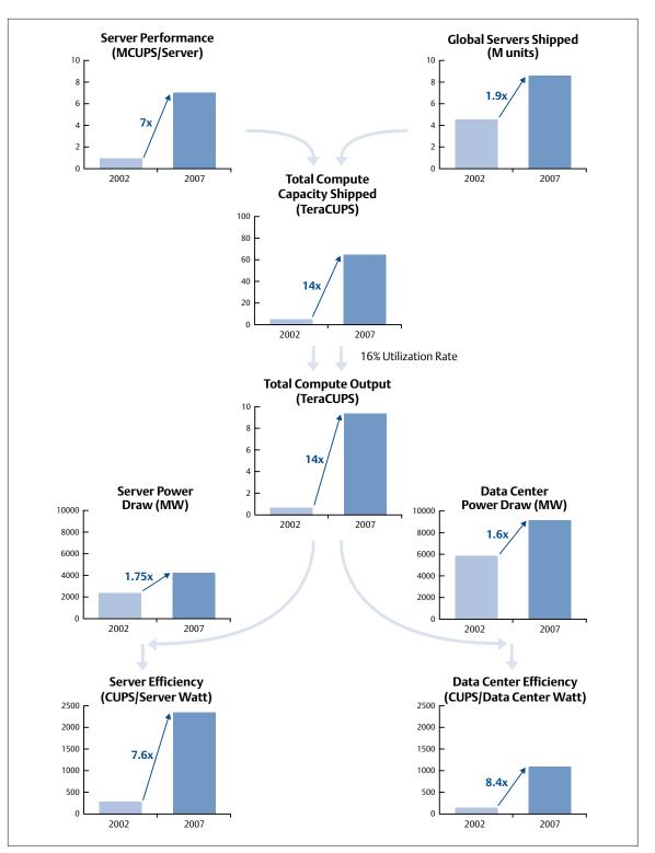
**Figure 6.** Once the 7:1 ratio between server performance in 2007 and 2002 was established, total server shipments and an assumed 16 percent utilization rate were applied to get an estimate of total TeraCUPS used in 2002 and 2007. This was then divided by server and data center power draw to determine the change in CUPS/Server Watt and CUPS/Data Center Watt between 2002 and 2007.
